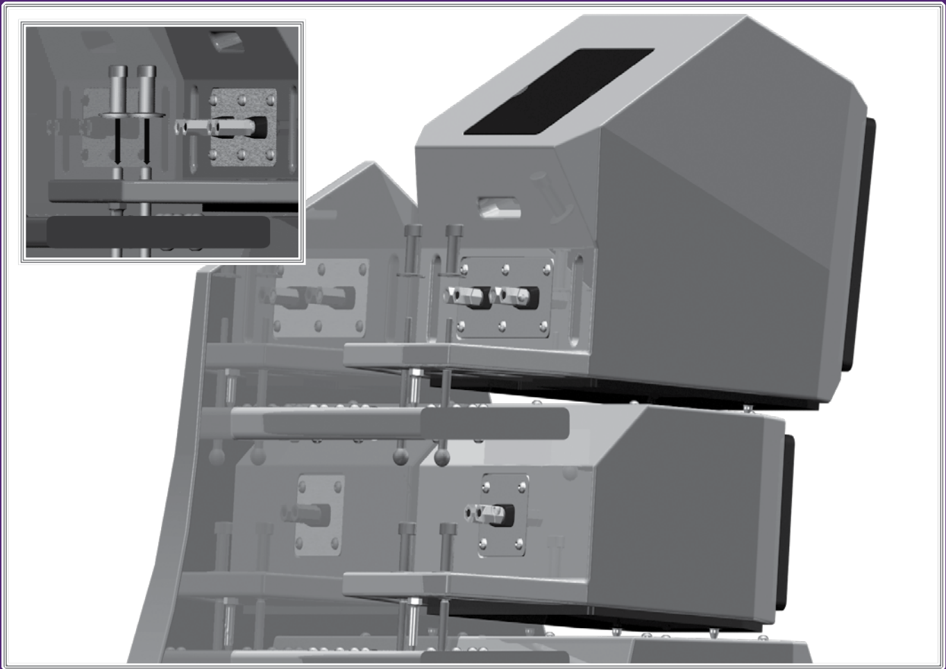
FIGURE 19 - INSTALL THE TETHER BOLTS. CUTAWAY OF X-2 SHOWING BOLT ASSEMBLY.
