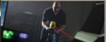
Laser Vibrometry Analysis, long used in automotive and aerospace applications, allows us to measure mechanical vibrations in our cabinets down to the level of nanometers. This invaluable data allows Wilson to optimize the composite structure of the cabinet, as well as the position and thickness of the internal braces.
