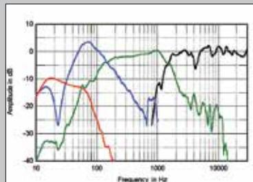
**Fig. 3** Wilson Alexia, acoustic crossover on listening axis at 50°, corrected for microphone response, with nearfield responses of: midrange unit (green), woofers (blue), port (red), respectively plotted below 350Hz, 1kHz, 300Hz.
