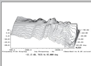
**Fig.5** Wilson Alexia, lateral response family at 50", normalized to response on listening axis, from back to front: differences in response 90-5° off axis, reference response, differences in response 5-90° off axis.
