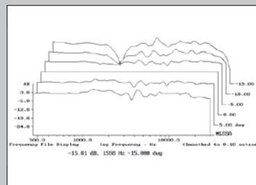
**Fig.6** Wilson Alexia, vertical response family at 50", normalized to response on listening axis, from back to front: differences in response 15-5° above axis, reference response, differences in response 5-10° below axis.
