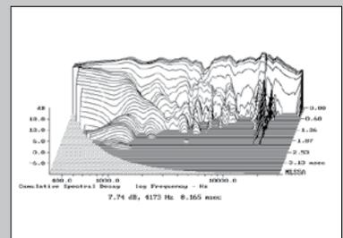
Fig.10 Wilson Alexia, cumulative spectral-decay plot on listening axis at 50” (0.15ms risetime).
