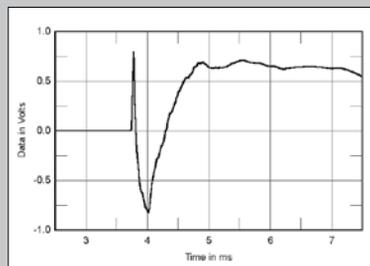
Fig.9 Wilson Alexia, step response on listening axis at 50” (5ms time window, 30kHz bandwidth).
