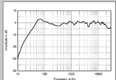
**Fig. 4** Wilson Alexia, anechoic response on listening axis at 50°, averaged across 30° horizontal window and corrected for microphone response, with complex sum of nearfield responses plotted below 300Hz.
