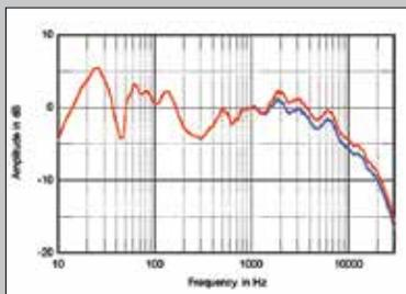
**Fig.7** Wilson Alexia, spatially averaged, 1/6-octave response in JA’s listening room with: original tweeter resistors (blue); new tweeter resistors (red). Note expanded vertical scale compared with fig.8.
