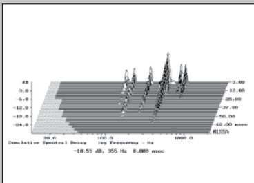
**Fig. 2** Wilson Alexia, cumulative spectral-decay plot calculated from output of accelerometer fastened to center of midrange-enclosure side panel (MLS driving voltage to speaker, 7.55V; measurement bandwidth, 2kHz).
