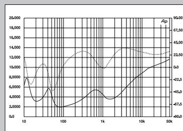
Fig.1 Wilson Alexia, electrical impedance (solid) and phase (dashed) (2 ohms/vertical div.).
