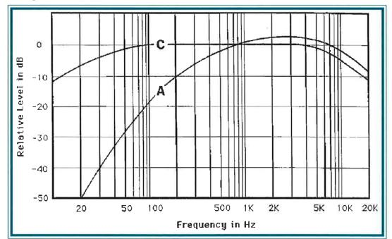
FIGURE 6.1 A & C METER WEIGHTING COMPARISON
