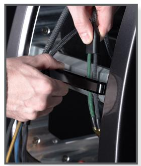
Note: It is extremely important to ensure the adjustable cable clamps are tightened. Failing to tighten the clamp compromises the gas-tight seal of the module. Hand-tightened to "snug" is sufficient.
