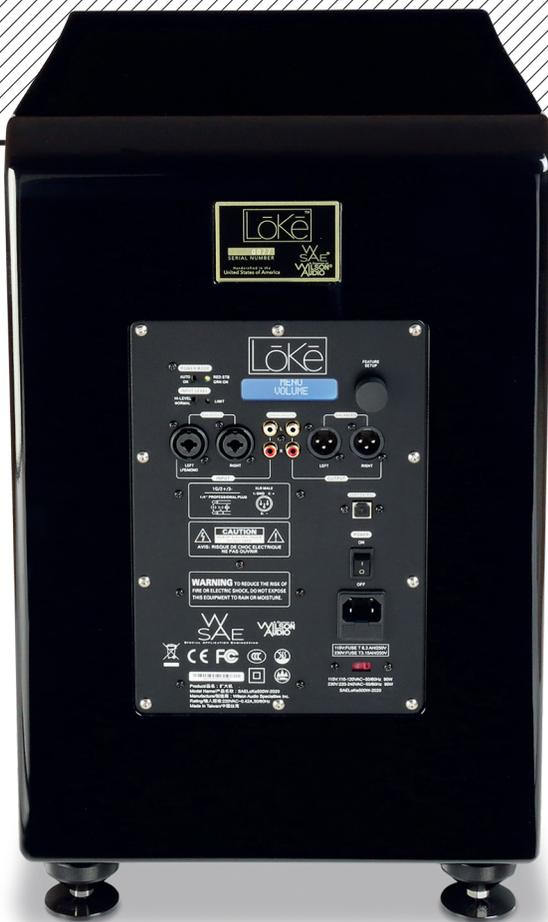
**LEFT:** Rear panel and OEM electronics are based on the 500W Dayton Audio SPA500DSP module with DSP menu and blue display. Single-ended (RCA) and high/low balanced (XLR) inputs are joined by filtered line outputs
