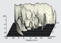
ABOVE: A resonance at the top of the mid unit's range (3kHz) is joined by a short-lived treble mode (14kHz)
