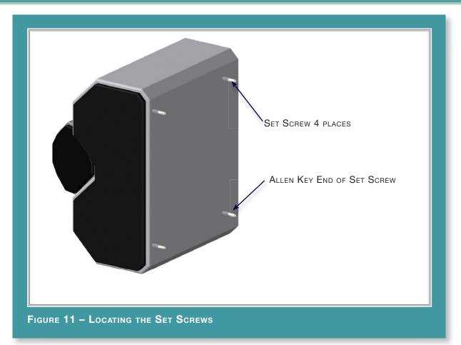
top of the Hourglass stand, but does not bolt to it. The setscrews sit inside the holes in the top of the stand.
