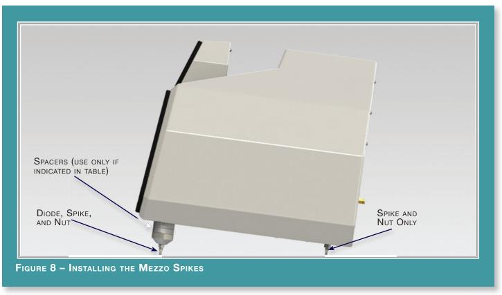
Note: the material used for the bottom of the Mezzo Wilson's proprietary high density composite X-material. While very hard, X-material is easily cross threaded when installing the spikes. Be careful that the spike thread is engaging properly into the bottom.
