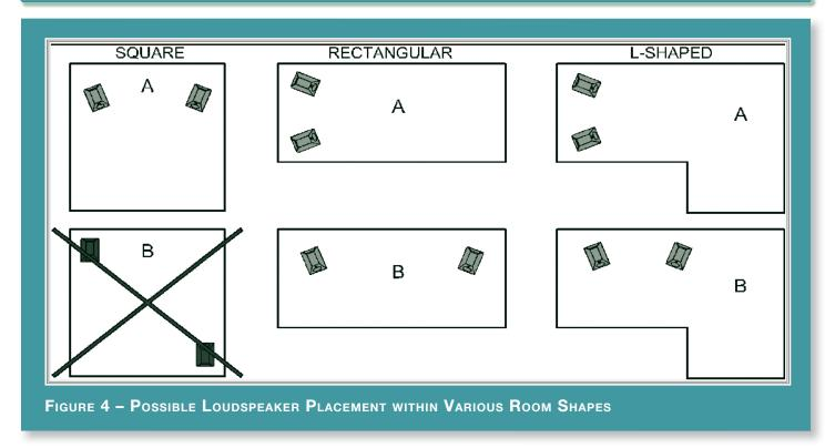
should fire from the end of the leg (short wall) toward the L, or they should be along the longest wall. In this way, both speakers are firing the same distance to the back wall. The asymmetry of the walls in L-shaped rooms resists the buildup of standing waves (see Figure 4).
