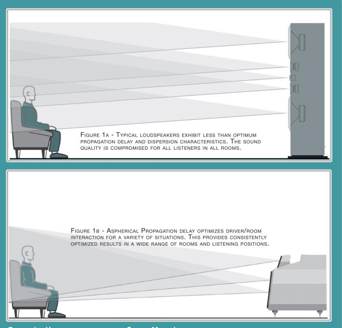
FIGURE 1 - USING TECHNOLOGY FROM SASHA, MEZZO'S GROUP DELAY IS CORRECTED IN THE TIME DOMAIN.
