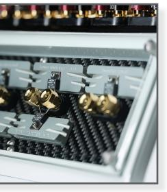
Woofer Module of your Chronosonic XVX, you may gain access to the resistor plate. These resistors serve several functions.
